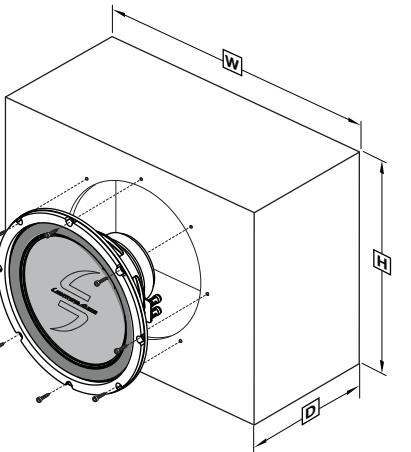
\*NOTE:  $V_b$  is NET volume (internal volume needed for woofer). Speaker, bracing and/or port displacement should be added to this volume. External dimensions are based on 3/4" (1.90cm) MDF.
